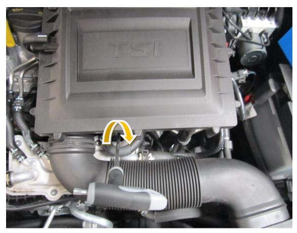
4. Locate the hose clamp at the rear of the airbox and remove.
