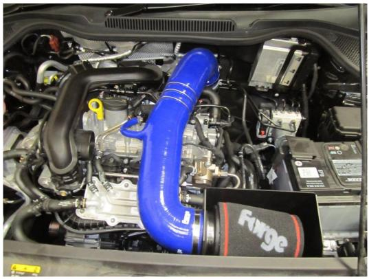
13. Remove the OEM breather hose and attach the new hose, do not over tighten the hose clamp as this could break the plastic OEM breather fitting.
